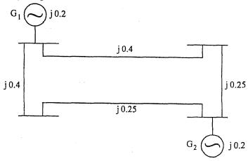
(b) Obtain Y<sub>br</sub>, Y<sub>loop</sub> by non-singular transformation method.
