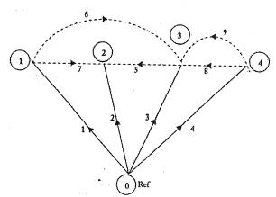
2. (a) Form the  $Y_{BUS}$  by using singular transformation for the network shown in Fig. below including the generator buses.
